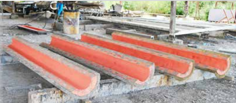
9 Rebound™ 25 was also used to capture intricate detail from the bark of a Banyan tree. Molds were used to make GFRG posts used to support the GFRG wall segments.
