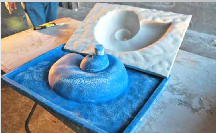
8 After 6 hours, the new sink is ready for installation. Mold Star™ 30 is ready to cast again.
