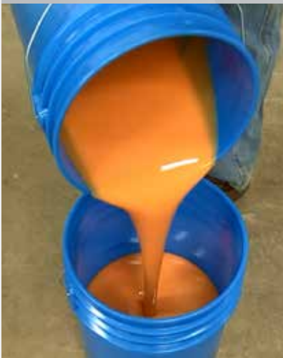
3 PMC™-780 is pigmented and drill mixed.
