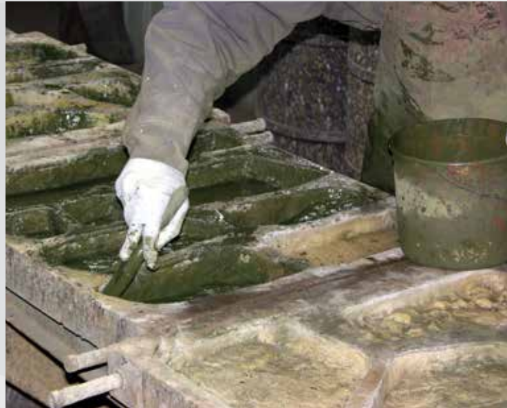
2 Mold cavity is pigmented to desired color.
