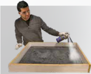
2 UNIVERSAL™ MOLD RELEASE IS APPLIED TO THE SEALED ORIGINAL MODEL
