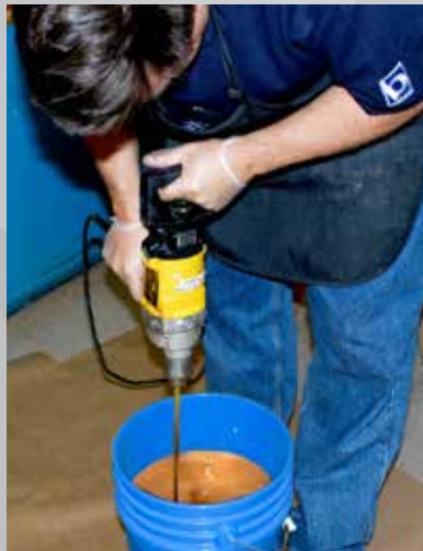
3 PMC™-780 is pigmented and drill mixed.
