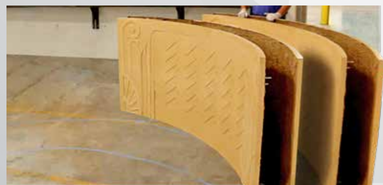
7 Four precast formwork panels are ready to ship to the job site.
