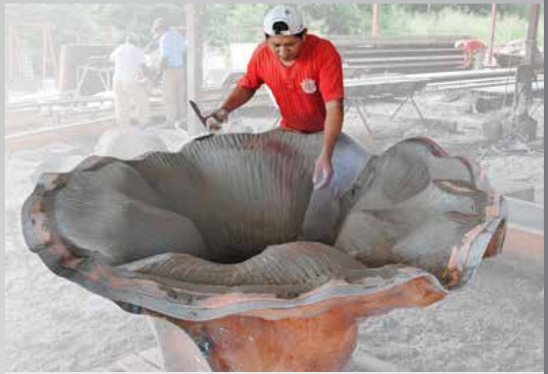
6 Mesh fiber and additional GFRC is hand applied to blend seams.
