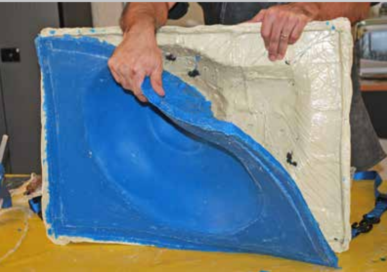
5 Mold Star™ 30 cures in 6 hours and the other half of the cavity mold is poured.
