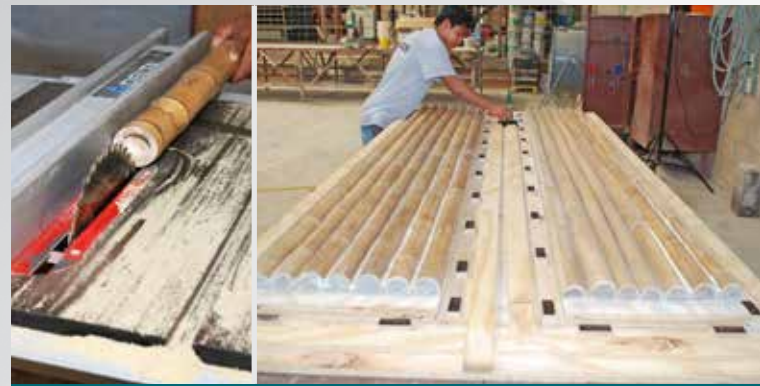
2 Half segments are stabilized and secured to table top. Registration keys were added around the model.
