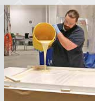
3 VytaFlex™ 60 is properly measured, mixed and poured over the entire model.
