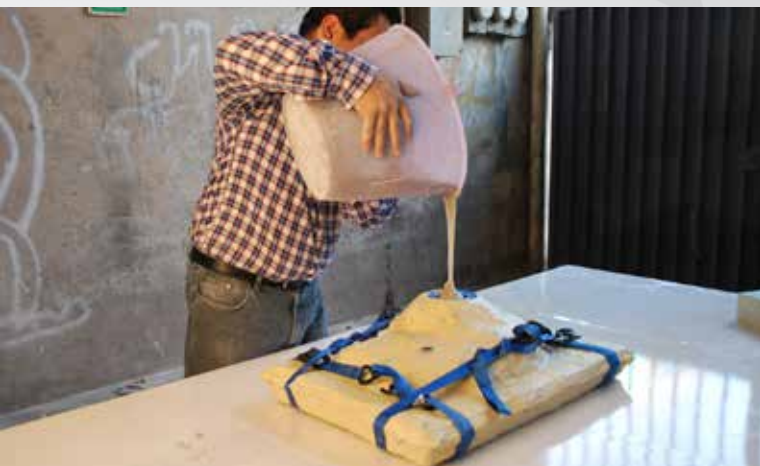
7 A low viscosity polymeric concrete is poured into the mold cavity.
