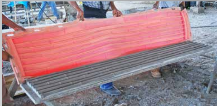
8 The GFRG panel reflects all of the detail of the original bamboo model. The concrete pieces can be stained for a realistic finish.
