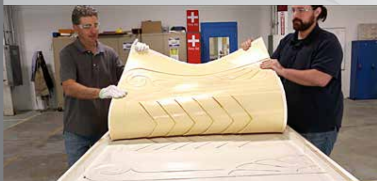
4 After curing for 16 hours, the rubber liner is demolded.
