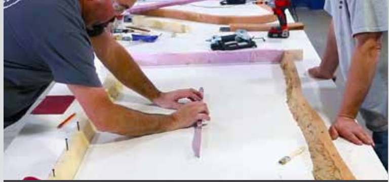
1 VytaFlex™ edge molds are screwed to a melamine surface. Cut foam is glued down to form the flame opening.
