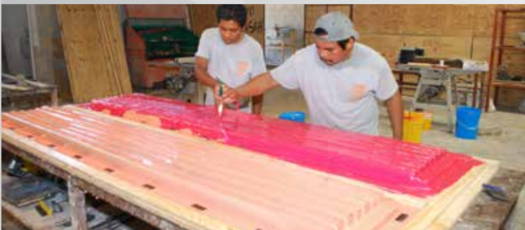
3 Three separate layers of Rebound™ 25 mold rubber are mixed & applied. Silc-Pig™ red pigment and Thi-Vex™ are added to ensure thorough coverage & fill deep areas.
