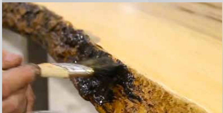
5 The edges are colored with Buddy Rhodes Glazes to simulate natural bark.
