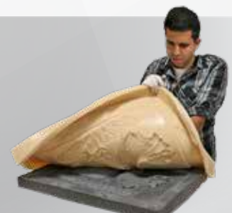
4 ORIGINAL IS DEMOLDED ONCE RUBBER IS FULLY CURED
