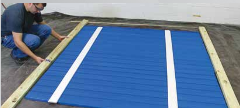
4 Mold will first be segmented to make four shower walls.
