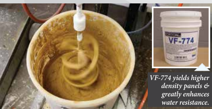
5 GFRC components are mixed in a high-shear mixer.
