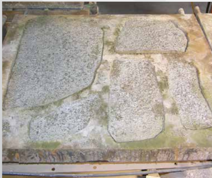
4 Concrete is allowed to set fully.
