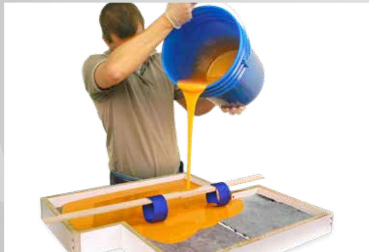
4 Rubber is poured onto the pavers, ensuring straps are embedded within the PMC™-780.
