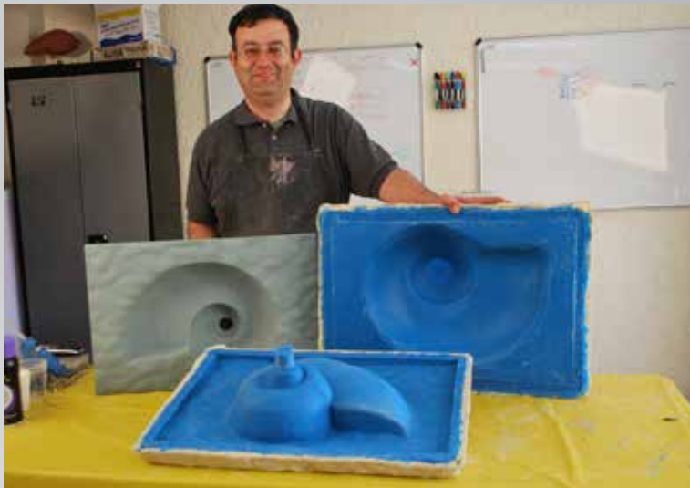
6 Mold Star™ 30 captures perfect detail and the mold is ready for polymeric concrete casting.
